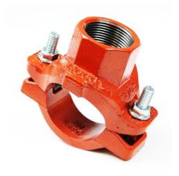
The Model 302 Mechanical Tee provides a fast and easy mid-pipe threaded branch outlet. It eliminates the need for welding or mulple fittings. The mechanical tee utilizes ductile iron housings, a grade E moulded gasket and heat-treated carbon steel track bolts and nuts. Pressure rated to 300 psi 20 bar.
