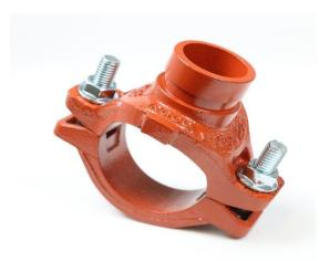
The Model 301 Mechanical Tee provides a fast and easy mid-pipe grooved branch outlet. The me-chanical tee utilizes ductile iron housings, a grade E gasket and heat-treated carbon steel track bolts and nuts. Maximum working pressure: 300 psi (20 bar.(
