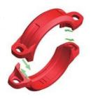
**T&G design:** The T&G (tongue & groove) mechanism provides a mechanical and frictional interlock resulting in a rigid joint which reduces undesired angular movement. W P T precision casting techniques allow the coupling segments to meet metal-to-metal when installed on properly grooved pipe.
