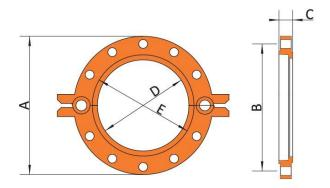
Flange Adapter allows for direct connection of a grooved system to ANSI class 125/150 flanged components
